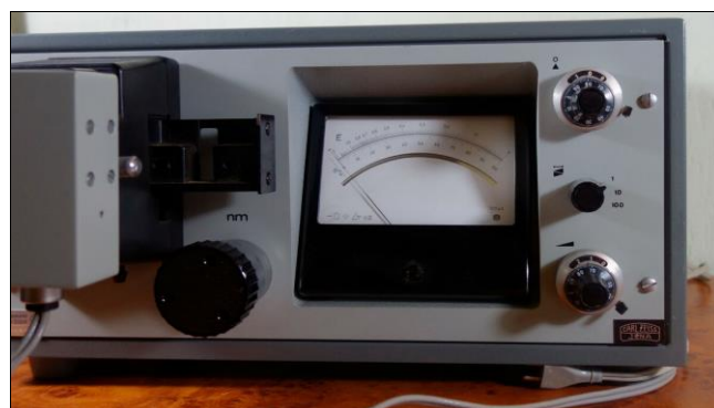
Fig 1: UR-20 Carl Zeiss Jena spectrometer
